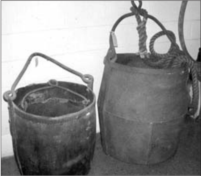
Many miner deaths were from accidents involving the "tub" or "bucket" that was lowered and raised from the underground mining areas. There were different sizes of these tubs. Pictured are some of the actual tubs used in area fluorspar mining. Men would stand in the tub with one leg on the inside and the other leg on the outside as to guide the tub and keep it from rubbing against the walls as it was lowered and raised. These tubs or buckets are on display at the Ben E. Clement Museum.
